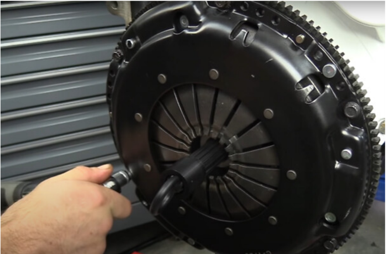
Consequence of not using the alignment tool during fitment
