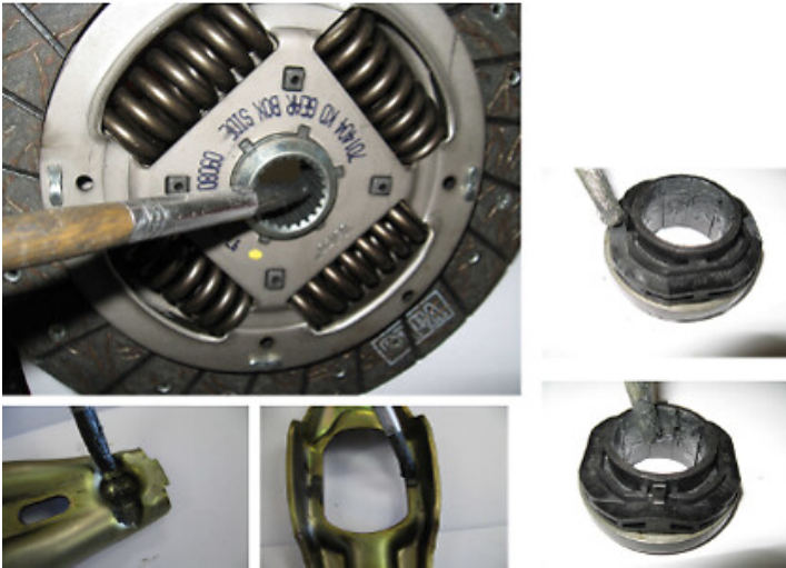
Lubricate the parts with only less amount of Grease. DONOT over grease
